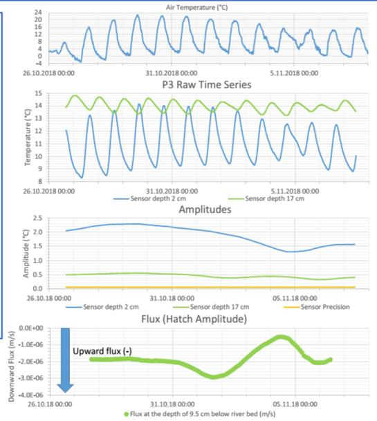
Figure 9 Vertical flow estimation @ location P3 (October 2018) using iButton vertical temperature profile data
