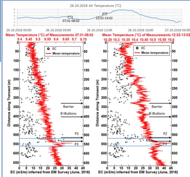
Figure 6 EC data inferred from EMI survey (June 2018), and mean temperature from DTS (26 Oct. 2018 @ 07:31-08:02 & @ 12:32-13:02)
