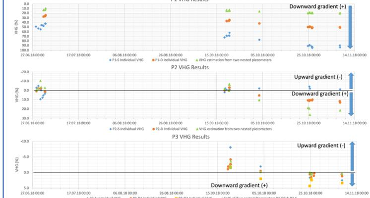
Figure 8 Vertical hydraulic gradient values from nested piezometers @ sites P1, P2 and P3 (see Fig. 5 for locations)
