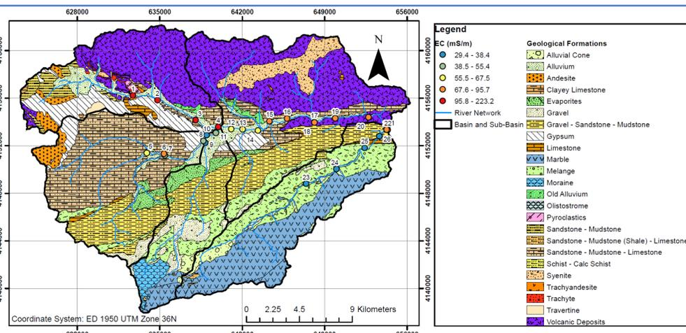
Figure 2 Geology of the basin. EC (mS/m) values are shown at sampling points
