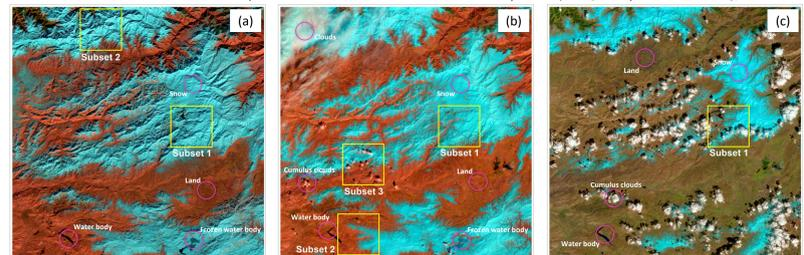
Figure 3. RGB false-color composite images of Sentinel 2 T37TFE tile for (a) Dec 2017, (b) Mar 2018, and (c) Apr 2018. R: Sentinel 2 Band 11 G: Sentinel 2 Band 8A B: Sentinel 2 Band 3 In this band combination, ice and snow appear as bright blue; whereas, water bodies are near black. Saturated soil can be seen also in blue, and clouds are still white.
