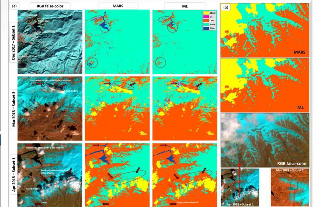
Figure 8. (a) The resultant classified images generated by MARS and ML, (b) Close-up view of April 2018 - Subset 1 image: The snow classification performance of MARS and ML, (c) Close-up view of March 2018 - Subset 2 image: Misclassification of snow as cloud at the snow-land boundary.
